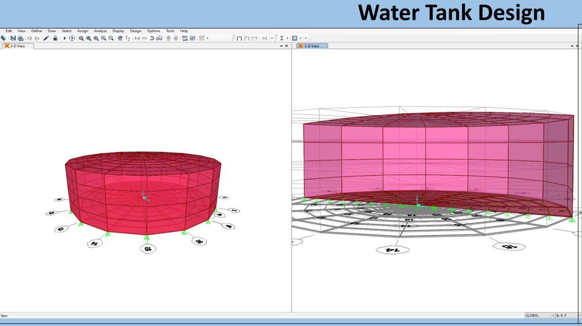
The water tank, which was designed by the program SAP 2000, will be developed using the standard of 200 gallons per person per day for the state of California and City of Corona standard of 4 people in a single-family household.
