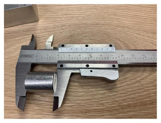
With the sample still in the caliper, this is a close-up view of the Vernier scale for easier reading.
