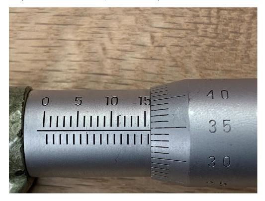
While the Vernier caliper's zero reading was truly zero (therefore no photo included), the micrometer was slightly off. This photo depicts the micrometer's zero reading.
