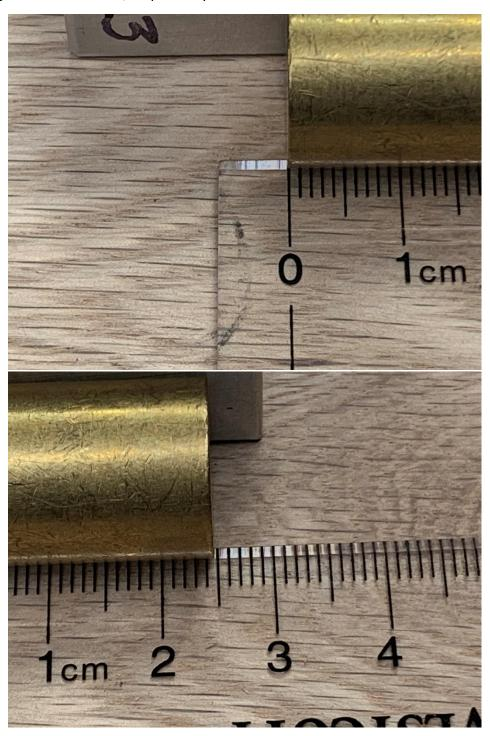
The following two photos depict the diameter measurement of the base of the cylindrical sample (left and right side).
