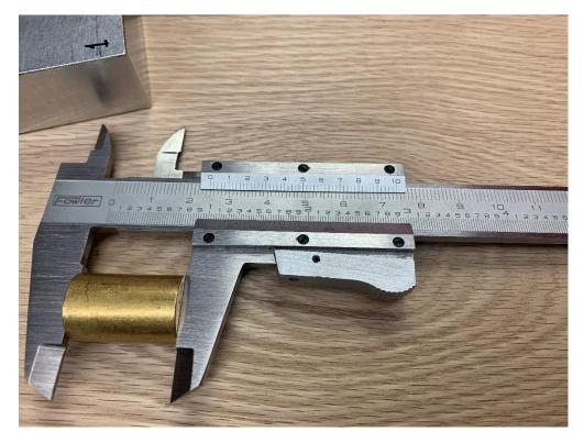
With the sample still in the caliper, this is a close-up view of the Vernier scale for easier reading.
