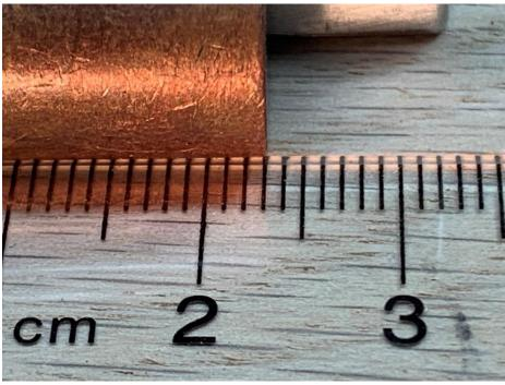
The following two photos depict the diameter measurement of the base of the cylindrical sample (left and right side).
