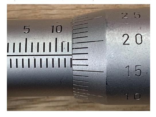
While the Vernier caliper's zero reading was truly zero (therefore no photo included), the micrometer was slightly off. This photo depicts the micrometer's zero reading.
