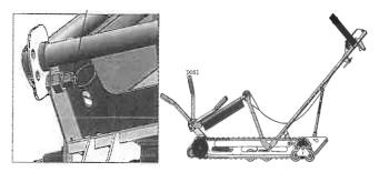
11. Unlock the Seat Latch by pushing down on the red Seat Latch Release Bar. Push down and forward on the Handle to fold Evacu-Trac closed.
