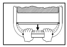
Do not try to lower the Front Auxiliary Wheels by pulling the Brake Release Bar without first pushing down on the Handle. This may stretch the Brake Cable.
