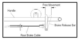
When you squeeze the Brake Release Bar it should travel until it just makes contact with the lime green Handle. This will allow you to comfortably hold Brake Release Bar in its released position when pushing The Evacu-Trac on flat surfaces or descending a stairway.
