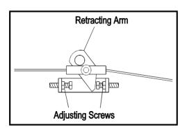
3. The final step is to ensure that the Track Parking Brake is functioning correctly. It is designed to stop and hold the rated load on the stairway. To do this, the Brake Spring must pull on the Brake Mechanism without any resistance from the Brake Cable. This can happen if the Front Brake Cable does not have sufficient slack.
