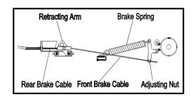
To check this, lay the open The Evacu-Trac on its side. Locate the Front Brake Cable. It should have approximately 19 mm (3/4 in) of slack, when measured vertically from the reference point shown in the drawing to the right.
