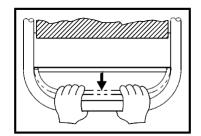
8. At landings, push down on the Handle and turn Evacu-Trac with all the weight on the Rear Auxiliary Wheels. Keep to the inside of the corner for maximum turning clearance. Align the machine at a right angle to the stairs and proceed down the next flight.
