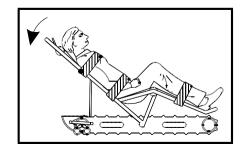
Then squeeze the Brake Release Bar with both hands. This will deploy the Front Auxiliary Wheels, making Evacu-Trac easier to push.
