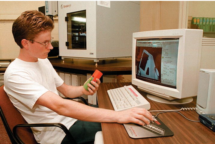
Rapid Pro lab: A grant from the National Science Foundation enabled the School of Engineering and Technology to acquire a Fused Deposition Model FDM 1600 Rapid Prototyping Machine. This high tech piece of equipment is able to build 3-D models and will be one of many exciting technologies available to our mechanical engineering and technology students in the Manufacturing and Robotics Laboratory, in the newly renovated Manufacturing Wing. This laboratory will house several industrial robots, a complete Computer Integrated Manufacturing (CIM) cell and computer hardware and software supporting CAD/CAM (computer-aided design/computer-aided manufacturing).
