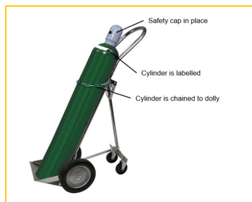
Figure 6-2: Proper gas cylinder transport.
