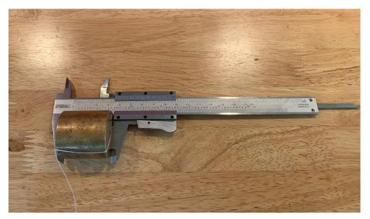
This is a close up to determine the ones and tenths place of the measurement. All that is needed is the location of the zero tick mark on the sliding scale.
