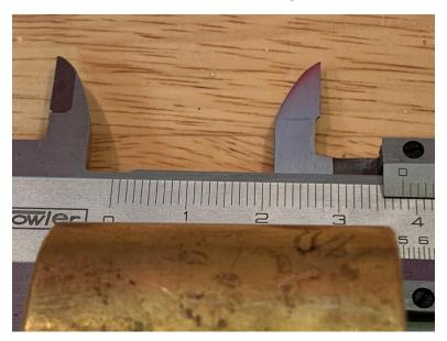
Here is a close up of the sliding scale to determine the hundredths and thousandths place of the measurement.
