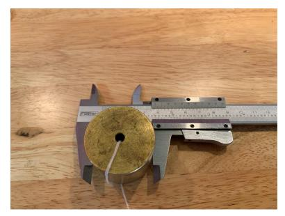
Use this photo to determine the ones and the tenths place of the measurement for D.
