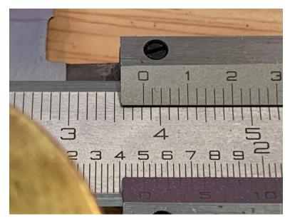
For an accurate reading of the sliding scale, use this close up and centered photograph (which avoids errors caused by parallax).
