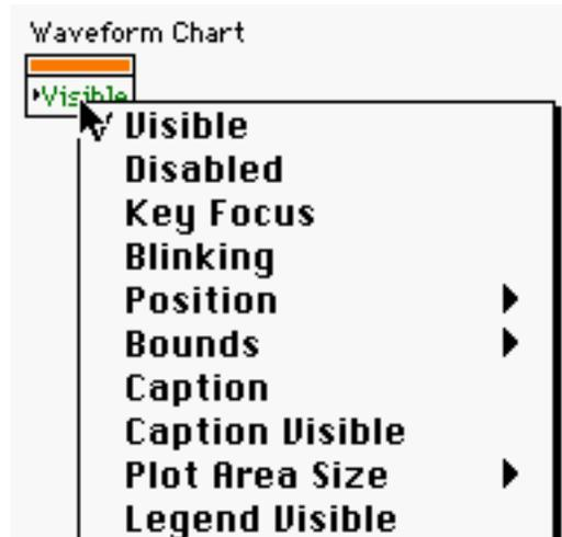
Figure 5.5 A partial list of options of the Attribute Node of the **Waveform Chart**
