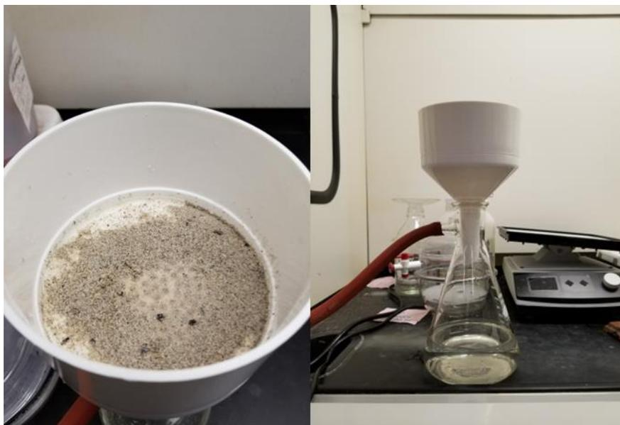
Figure 7. Top view of potential microplastics (left) and bottom view of reusable saturated NaCl solution (right).
