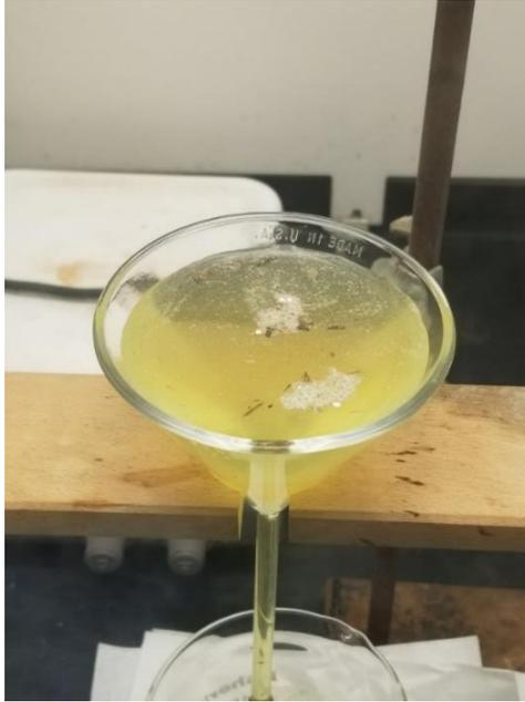
Figure 9. Density separation after digestion.
