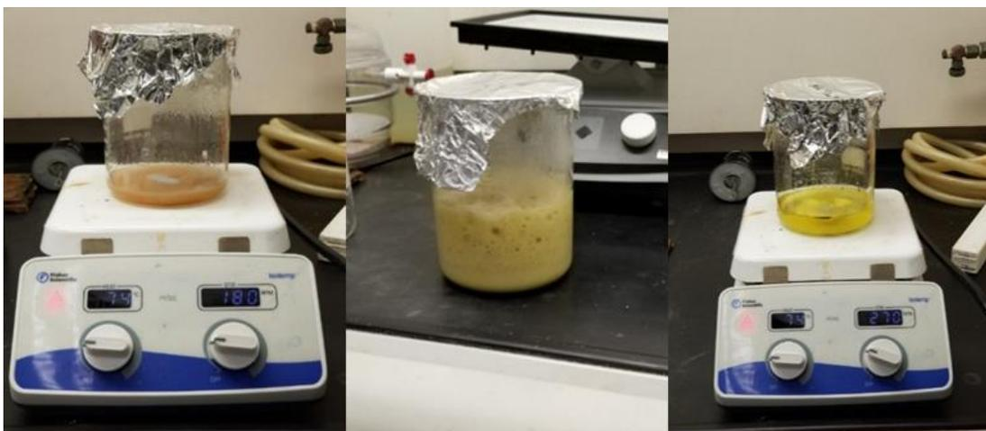
Figure 8. Wet Peroxide Oxidation: Before oxidation (left), generation of hydroxyl radicals (middle), and after oxidation with NaCl pellets (right).
