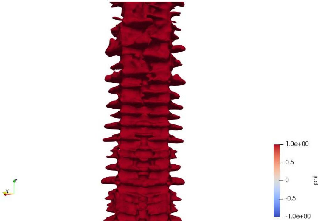
Figure 41: Case 2: 292,951,724 iterations (36.6 seconds) simulation output of Phi measuring the upper limit and exhibiting tertiary dendrites.
