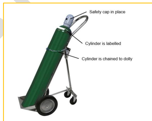
Figure 6-2: Proper gas cylinder transport.
