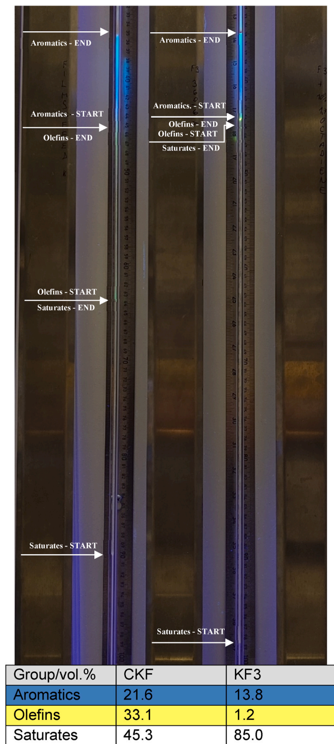
Fig. 4. FIA analysis of chosen samples – CKF = kerosene fraction of crude pyrolysis oil from films (left); KF3 – kerosene fraction from pyrolysis oil from PE films after hydrotreatment at 360 °C and 6 MPa (right). Reproduced with permission from Ref. [15] Copyright 2024 Elsevier.
