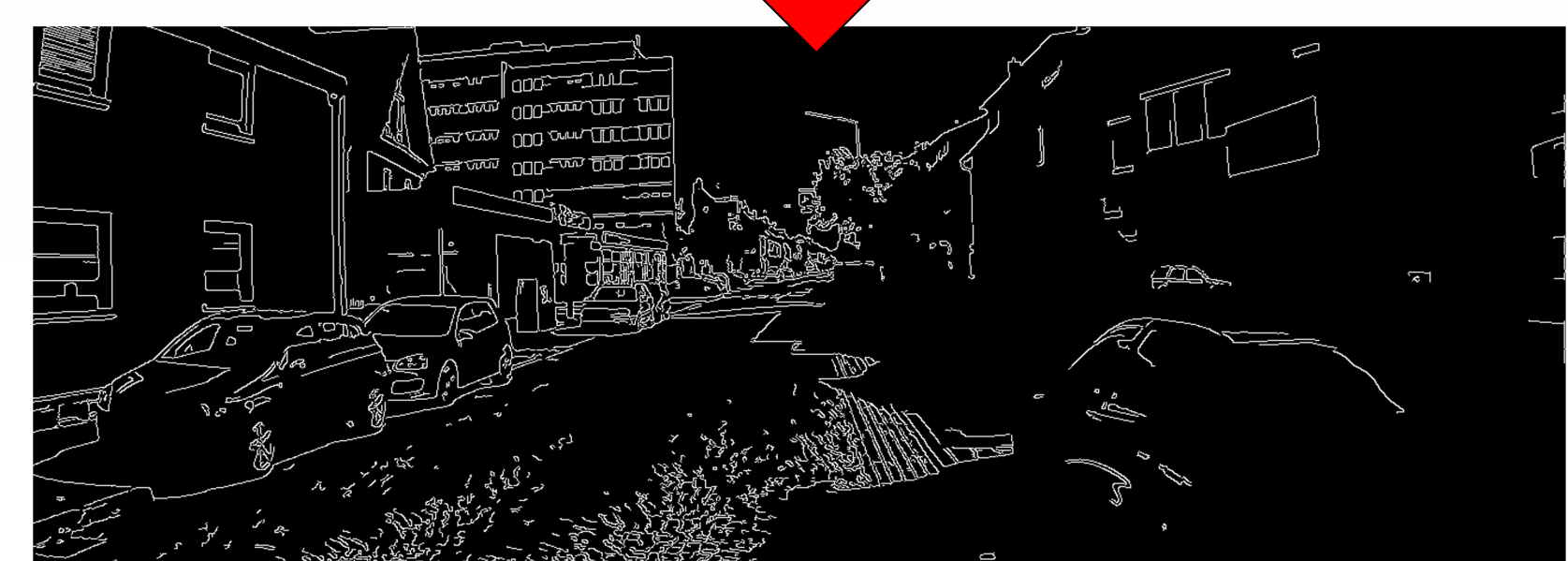
Sample of the conversion from video frame to an edge detection frame.
