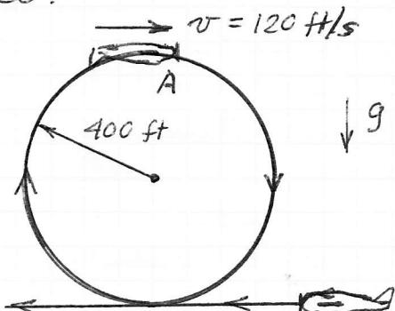
$$\begin{array}{c} N \\ \downarrow \\ mg = 150 \text{ lb} \end{array} = \begin{array}{c} F \\ \downarrow \\ ma_n \end{array}$$
