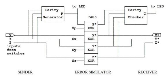
Since PXYZ patterns are to be sent with EVEN parity, the parity generator will examine the input pattern XYZ and output a 1 if the pattern has the wrong parity (ODD), and a 0 otherwise. Thus, if inputs XYZ = 100 (odd parity), then P = 1. The transmitted pattern will be PXYZ = 1100, with even parity as required. Again, the parity generator is to be designed with XOR's <u>only</u>.
