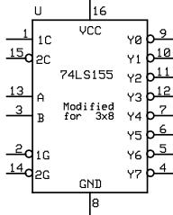
74LS155 has active-low outputs as indicated by the bubbles on the output pins Y0 through Y7.
