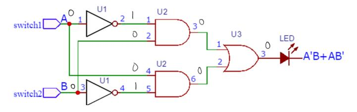
Step 3, set the inputs A and B both to zero. Step 4, starting at the output, use the logic probe to work backwards tracing the incorrect values. Using the logic probe, you can verify the output of the circuit, pin 3 of U3, is 1 instead of 0. Checking the inputs to that gate (which are easy to identify from the wiring diagram), check pins 1 and 2 of U3. You will discover that pin 2 of U3 is a 1 instead of the expected value of 0 as shown in the figure below:
