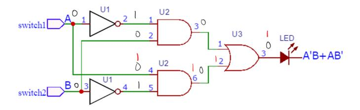
Now check the connection between pin 4 of U2 and the switch driving A (or pin1 of U1). You have discovered the bug! As indicated in the figure below, Pin 4 of U2 is connected to pin 2 of U1 instead of pin 1 of U1.
