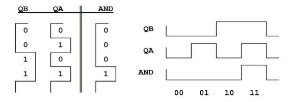
**3.3\*** Notice that the waveforms are just a graphical form of the truth table (rotated 90 degrees counter clockwise). By displaying such waveforms on a scope, you can obtain a description of circuit behavior equivalent to a truth table.
