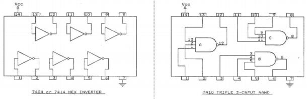
For each logic function, draw the wiring diagram of the logic gate (include the pin numbers) in your lab manual. As before, you do not have to redraw the 7493 counter for each wiring diagram. Just label the inputs of the gates with the appropriate Q output from the counter. For each logic function draw the waveforms of the msb (most significant input bit) and the output of the respective gate and verify that the output matches your truth table values from section 3.1.
