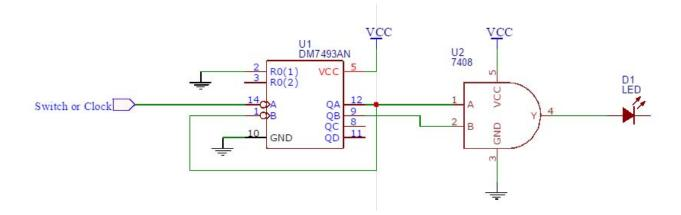
Connect QB and QA to two inputs of a 7408 AND gate. (Don't forget 5V and ground connections; pins 14 and 7. If you forget, the chip is inactive). Referring to the truth tables in 3.1, Y = QB and X = QA. Connect the clock A input of the counter (pin 14) to the normally high pulser (pushbutton switch). Connect QB, QA, and the output of the AND gate to LEDs and verify that the correct outputs are produced by referring to the truth table below (or your answer to part 3.1).
