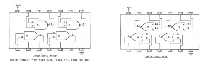
For each logic function, draw the wiring diagram of the logic gate (include the pin numbers) in your lab manual. You do not have to redraw the 7493 counter for each wiring diagram. Just label the inputs of the gates QA and QB. For each logic function draw the waveforms of QB and the output of the respective gate and verify that the output matches your truth table values from section 3.1.
