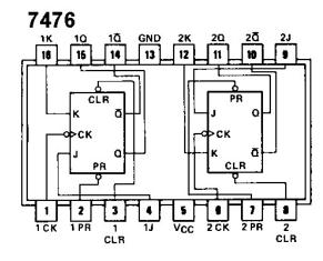
Referring to the 7476 pin assignments above, draw a wiring diagram to test the behavior of a JK flip-flop.
