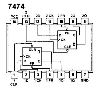
• In the wiring diagram, connect the D input to one of the toggle switches and connect the Q output to one of the LEDs and Q' to another LED.
