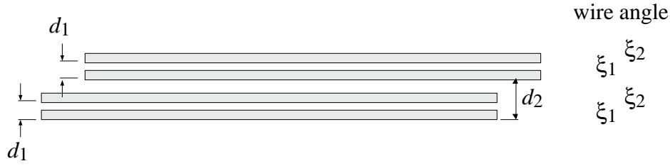
Figure 4.5: Configuration of the wire chamber package.
